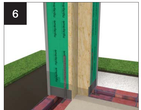
6 Fit straps and or structural anchors
