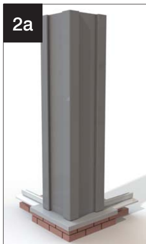
Claddings with masonry plinth cap
