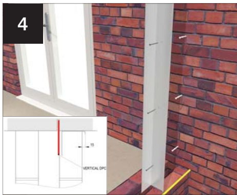
4 Drill abutment bracket. Mark position of bracket 50mm down from eaves height (see fig 5). Fix abutment bracket to the host wall using appropriate anchors (not supplied). NOTE: THE ABUTMENT BRACKET MUST BE SET 15MM OUTBOARD OF THE BUILDING LINE AS SHOWN. Fit DPC.
