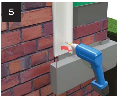
5 Position cladding clip around column and into slot in brickwork. Drill through hole and mark brickwork. Plug and screw. Screw along length of the column
