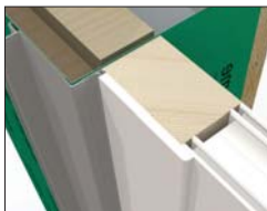
Pack detail shown between column and full height frame or door when using brick plinths.
