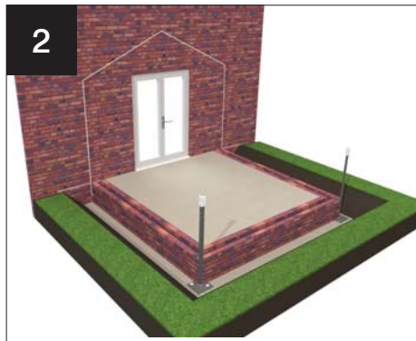
2 Complete base to slab level
