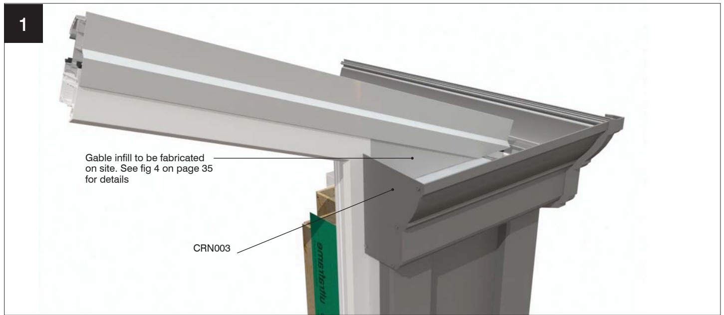
External view of short return gable with Cornice
