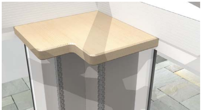
Timber Cap - exact finish at fitters discretion
