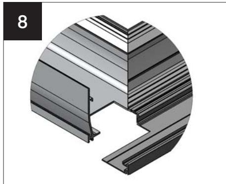
Standard eaves with 165mm boxgutter.
