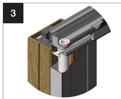
Cornice shown in situ with concealed downpipe
