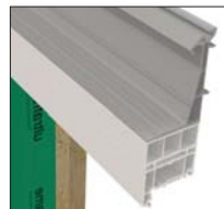
A 30mm (minimum) add on required if specifying LivingRoom (below fascia). Add on only required between columns. NOTE: DO NOT RUN ADD ONS ONTO OR OVER THE COLUMN
