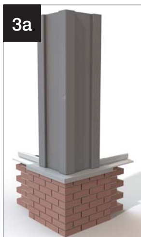
Claddings with masonry plinth cap (on dwarf wall)
