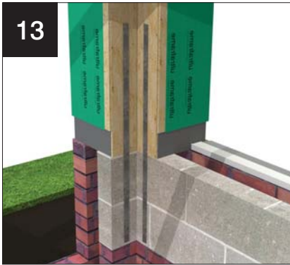
13 LARGE 90° CORNER Fasten straps down inside of walls of large 90° corner column
