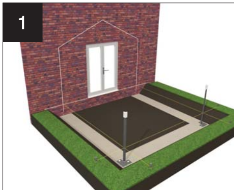
1 Fix brickwork set out posts to footings, align to stringline
