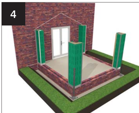
4 Fit abutment columns
