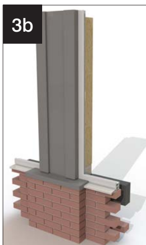
Claddings with masonry plinth cap (on dwarf wall)
