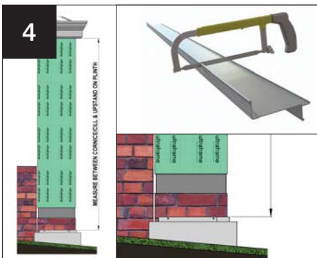
4 Measure between the underside of Cornice or cill and the top of the upstand on the plinth. Cut the cladding clips to this measurement. IMAGE SHOWS GROUND RE-INSTATED (SLOPED)
