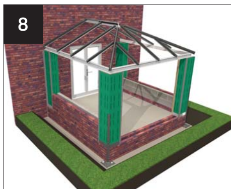
8 If dwarf walls are required, build up walls and tie into columns
