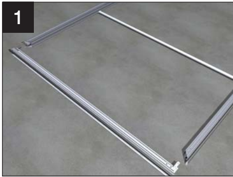
1 Layout the pieces of the lantern eaves beam.
