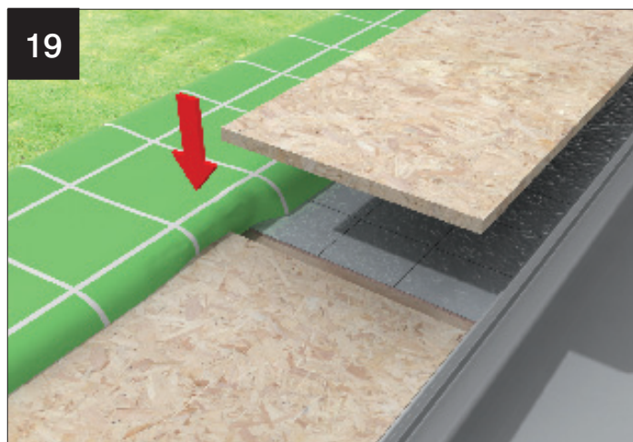
Fit the pre-cut 18mm plywood top panels and screw down to the noggins
