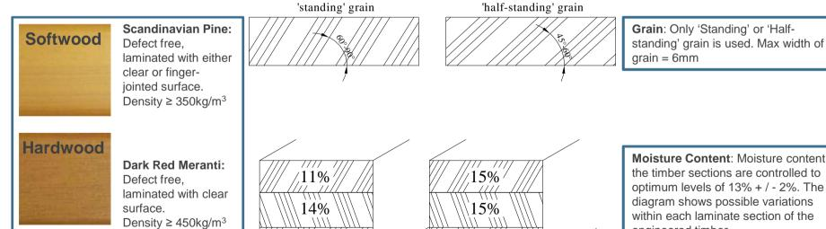
Moisture Content: Moisture content of the timber sections are controlled to optimum levels of 13% + / - 2%. The diagram shows possible variations within each laminate section of the engineered timber.
