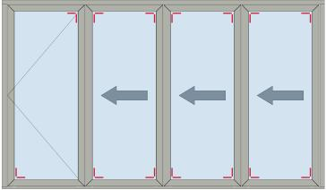
Master Door 1st Sliding Door/ 2nd Sliding Door 3rd Sliding Door Keep Door
